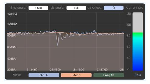
**Graph** – Displays the historical loudness data measured. This image can be placed on a UCI for convenient real-time viewing. The colors of the graph can be customized in the plugin properties.
